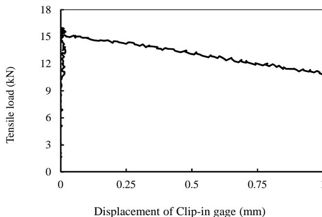
Fig. 1 Direct tensile load-displacement relationships of UHPFRC (Choi et al. 2012)
