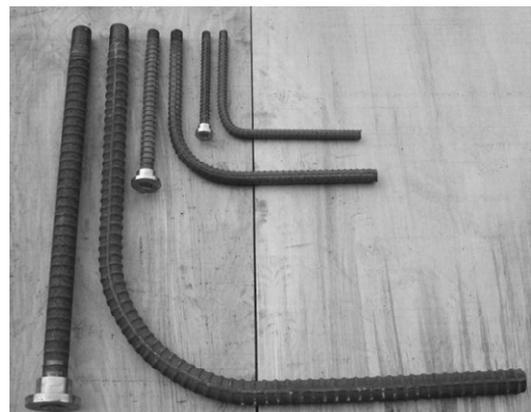
Fig. 2 Headed and hooked bars
