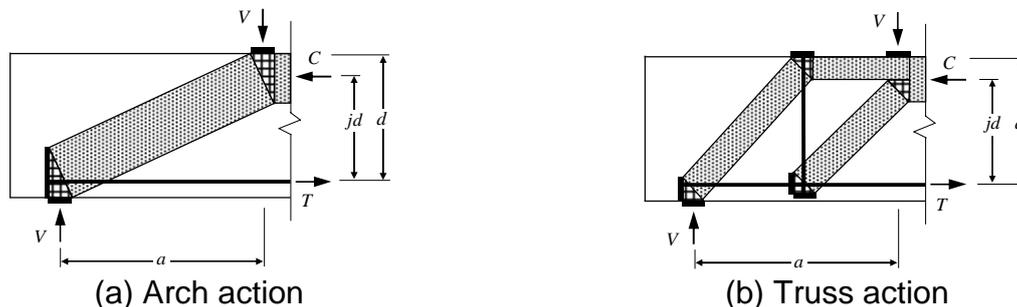
Fig. 1- Shear transfer mechanisms of deep beam: (a) Arch action; (b) Truss action
