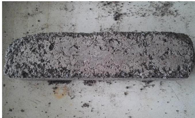
Fig. 4 External appearances of sand-fixing material after certain freeze-thaw cycles
