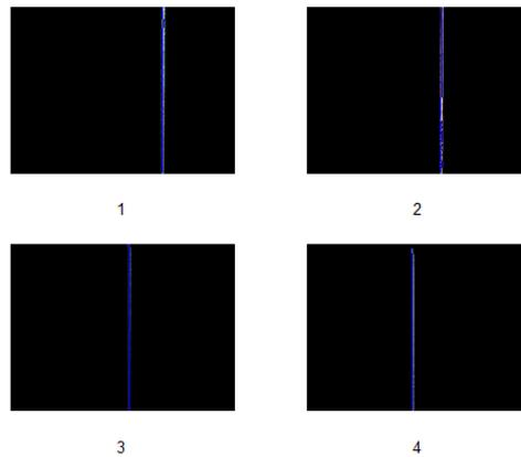
Fig. 4 Laser line moving process on camera imaging plane
