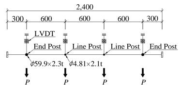
Fig. 1 Floor plan of fence support system
