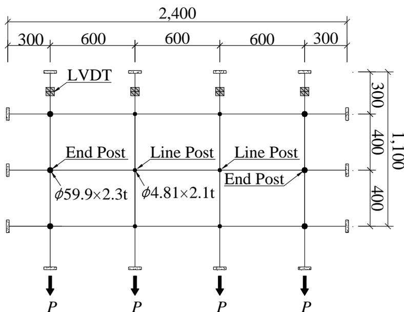
Fig. 2 Floor plan of matrix support system
