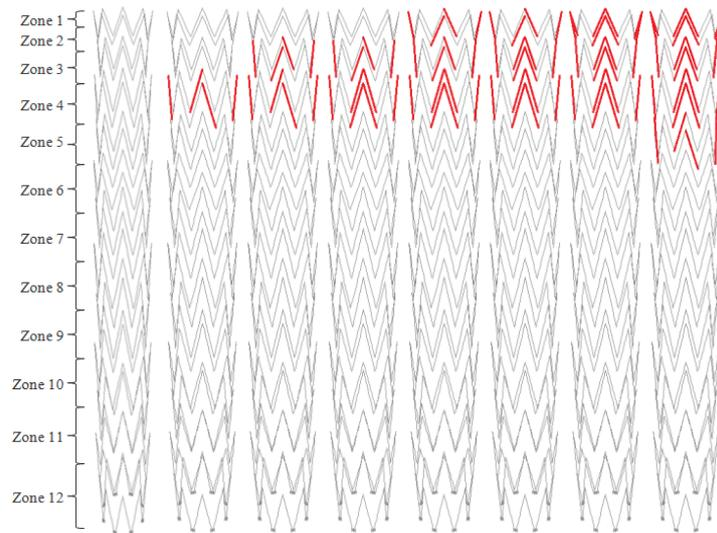
Fig. 7: Positions of Dampers for Each Option
