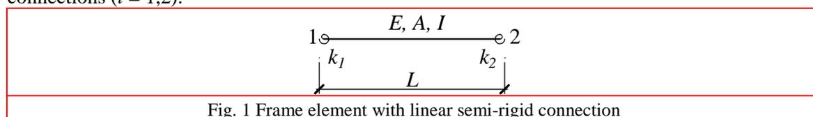
Fig. 1 Frame element with linear semi-rigid connection
