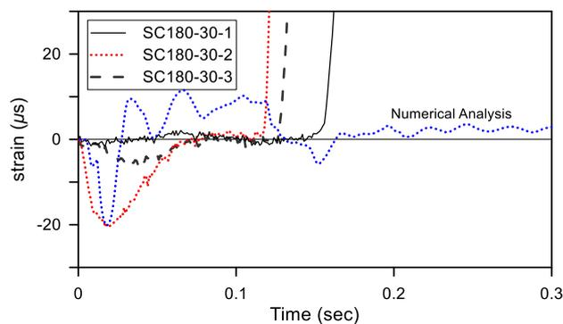
Fig. 4 Strain histories of experiment and numerical analysis
