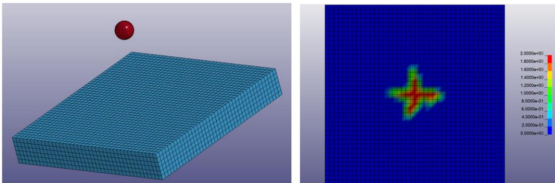
Fig. 3 Modeling (Left) and contours of strain on rear face of UHPC (Right)
