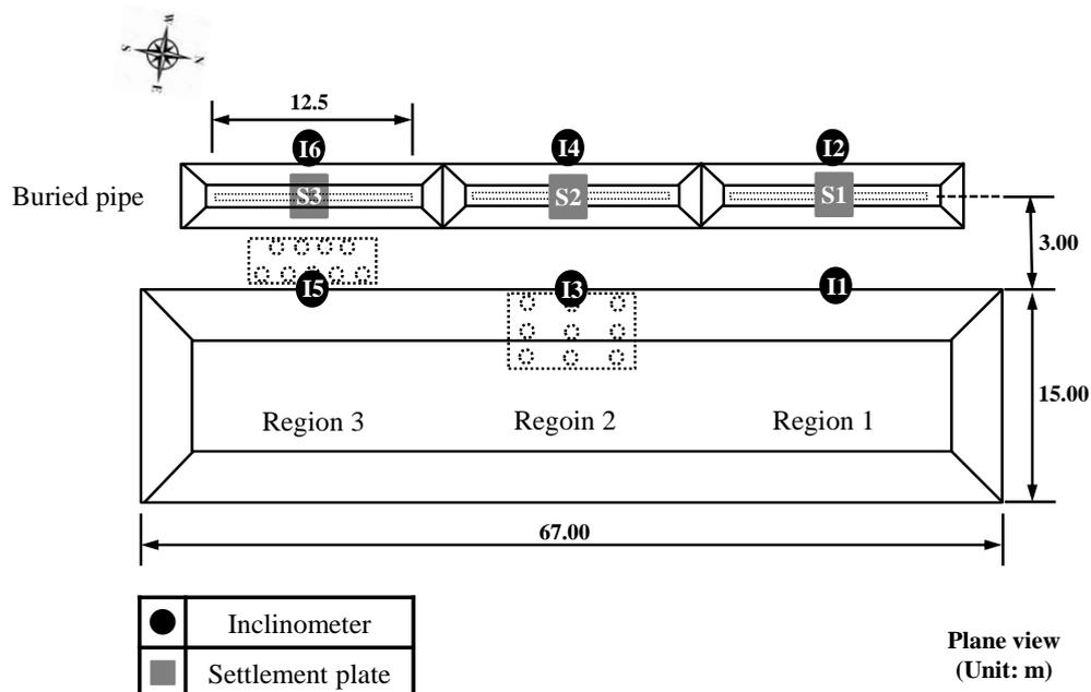
Fig. 4 Plane view of full-scale test on embankment
