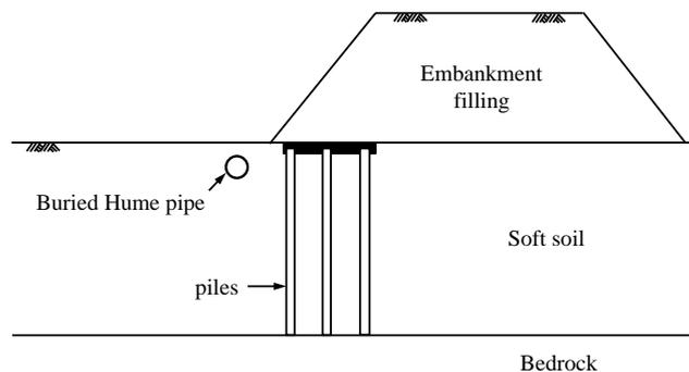
Fig. 2 Pile-supported embankment
