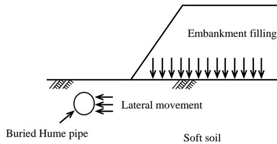
Fig. 1 Buried Hume pipe subject to lateral flow of soft soil caused by embankment filling
