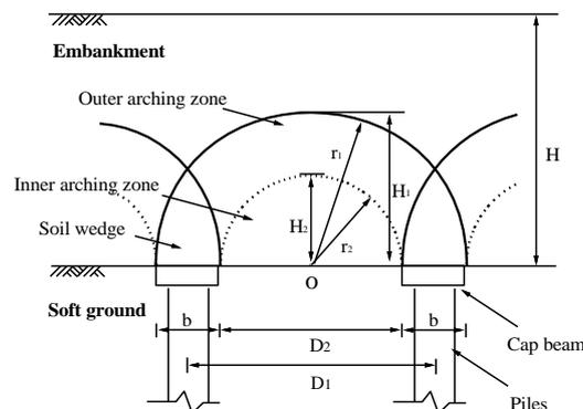
Fig. 3 Soil arching mechanism (Hong et al. 2007)
