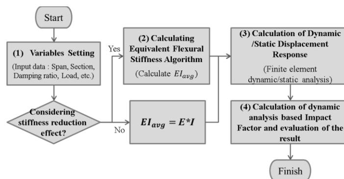
Fig. 2 The MATLAB program's flowchart
