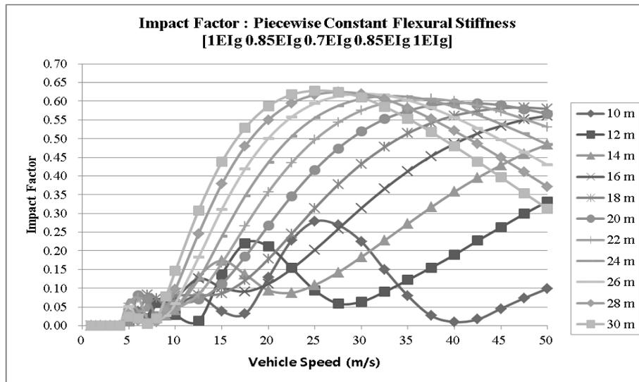
Fig. 3 Impact Factor : Piecewise constant flexural stiffness (cracked bridge) [1EI<sub>g</sub> 0.85EI<sub>g</sub> 0.7EI<sub>g</sub> 0.85EI<sub>g</sub> 1EI<sub>g</sub>]
