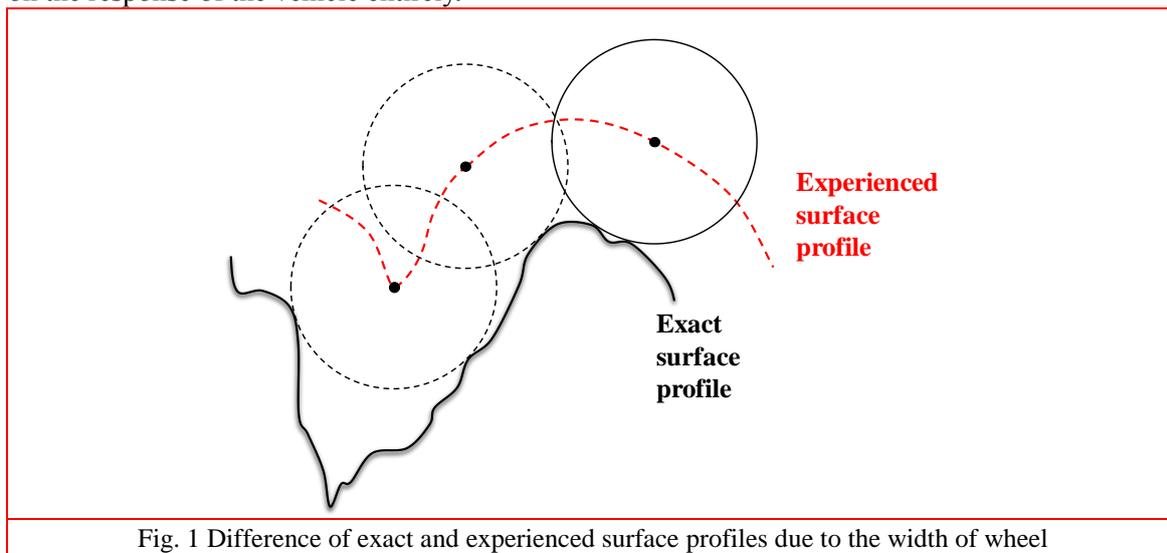
Fig. 1 Difference of exact and experienced surface profiles due to the width of wheel
