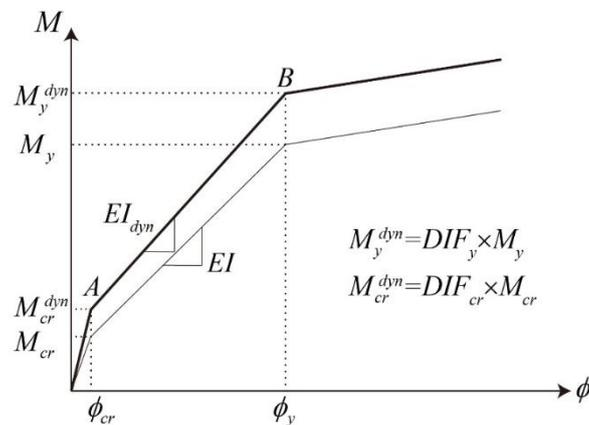
Fig 1. Moment-curvature relationship considering dynamic increase factor
