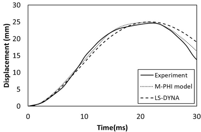
Fig. 2 Displacement history for RC1-2 at mid span
