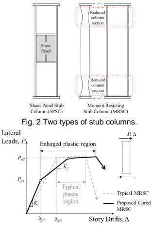
Fig. 3 Strength backbone curves of hysteretic behaviors of typical and proposed cored MRSCs.
