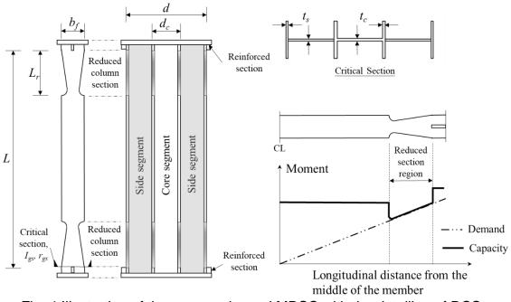
Fig. 4 Illustration of the proposed cored MRSC with the detailing of RCSs.
