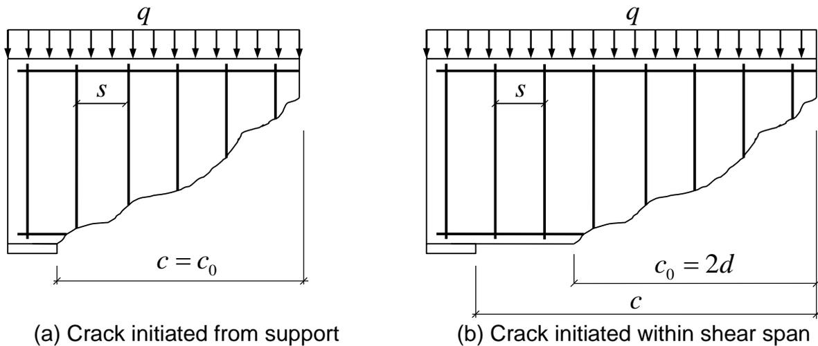
Fig. 1 Description of possible failure planes in PMR approach
