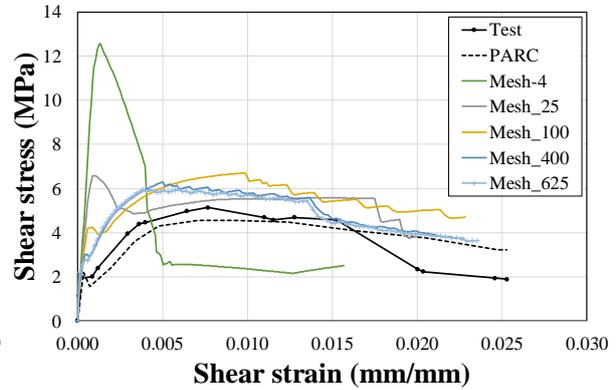
(b) With rotating crack model
