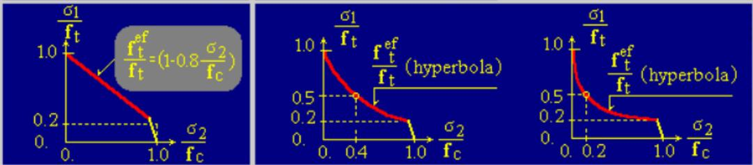
(b) Tension-compression failure function for concrete
