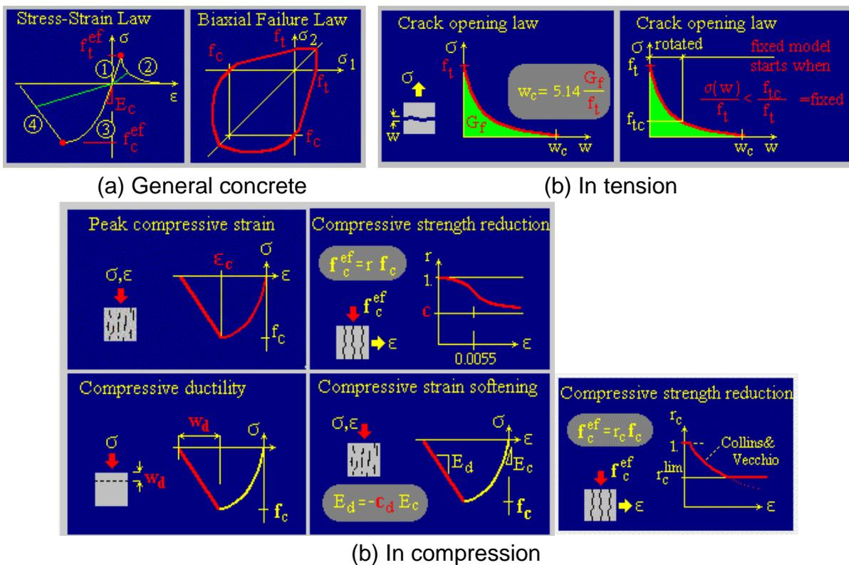
Fig. 2 CCSBETA for concrete material
