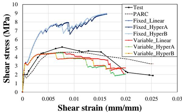
(c) With fixed crack model
