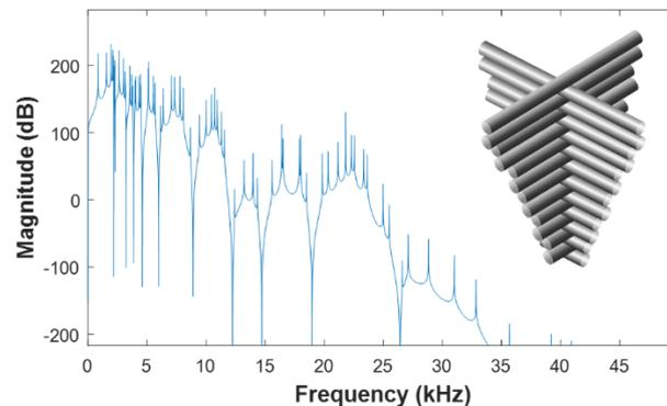
Fig. 3 Frequency response function (FRF) of the combined chain of six different homogeneous chains consisting of 100 mm, 90 mm, 80 mm, 70 mm, 60 mm, 50 mm cylinders, respectively. The inset show schematic diagram of the combined chain.
