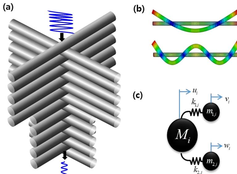
Fig. 1 (a) schematic diagram of the combined cylinder chain, (b) 1<sup>st</sup> and 3<sup>rd</sup> bending vibration mode of a slender cylinder, and (c) discrete element model (DEM) of a cylinder taking into account two vibration modes.
