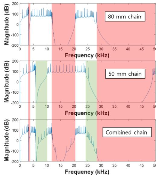
Fig. 2 Frequency response function (FRF) of a 80 mm chain model (top), 50 mm chain model (middle), and combined chain model (bottom)
