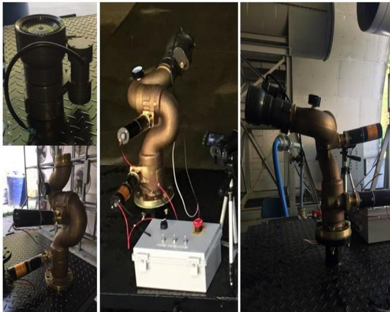
Fig. 3 Automatic monitor system
