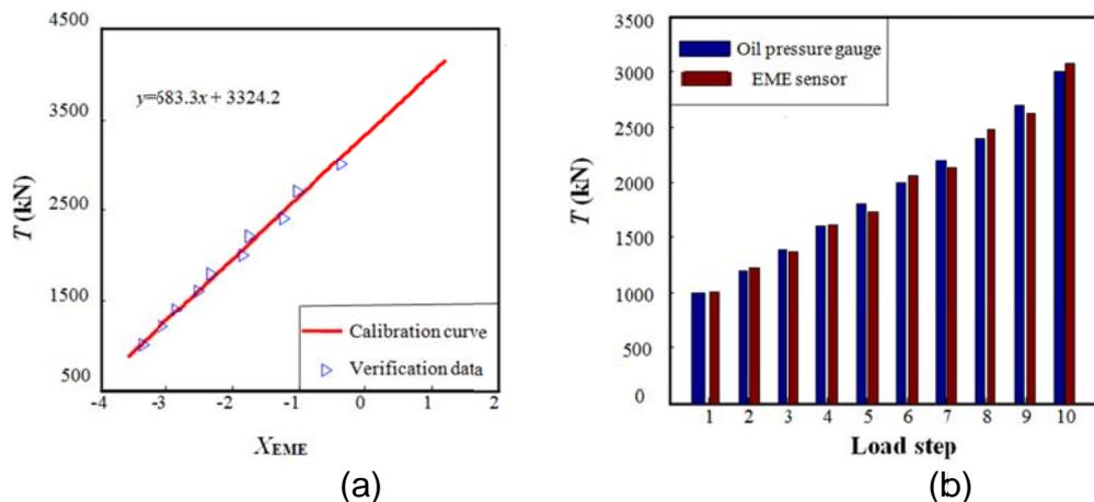
Fig. 5 The results of in-situ verification. (a) Calibration curve and verification data, and (b) The compared results of EME sensors with the oil pressure gauge.
