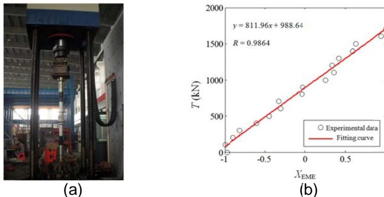
Fig. 2 The full-scale experiment on large steel cables. (a) Experimental setup, and (b) Experimental result.
