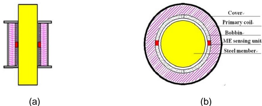
Fig. 1 Structure of an EME sensor. (a) Vertical section view, and (b) Cross-section view.
