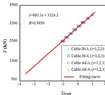
Fig. 3 Results of factory calibration for the typical steel cable PES(C)7-151.
