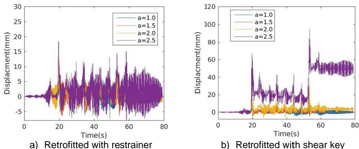
Fig. 7 Transversal displacements of bridge piers retrofitted with different devices
