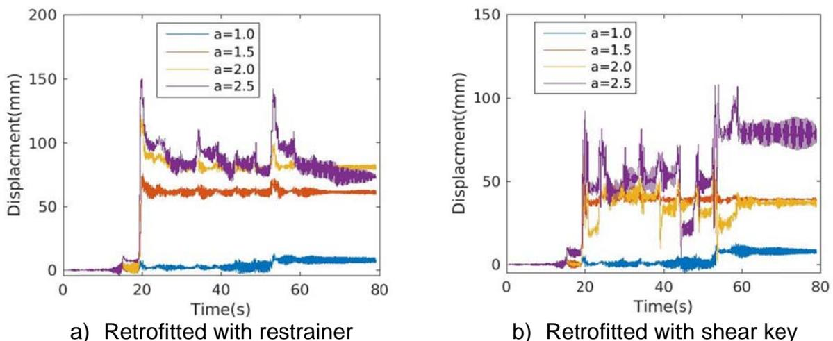
Fig. 6 Transversal displacements of bridge decks retrofitted with different devices
