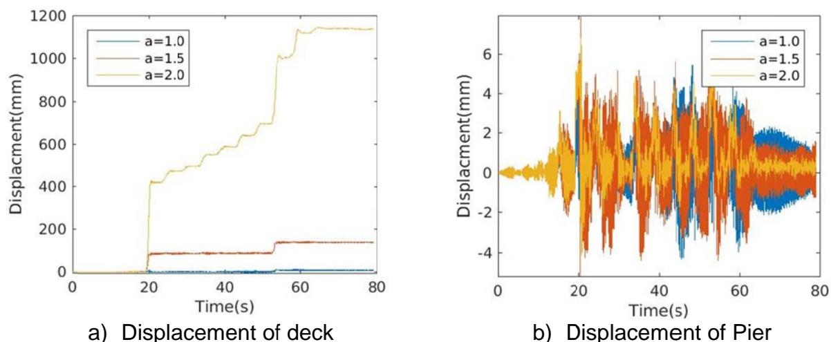
**Fig. 4** Transversal displacement of bridges without additional constraint
