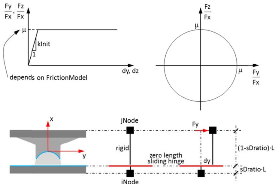
Fig. 2 Flat slider bearing element in OpenSees
