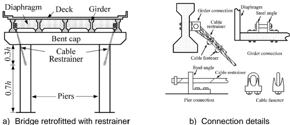
Fig. 5 Configuration of cable restrainer
