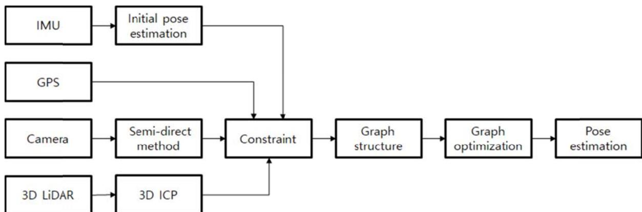
Fig. 1 Overall flow diagram of the proposed method.
