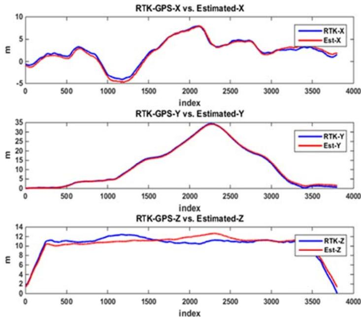
**Fig. 5** Localization results. The red solid line indicates the estimated pose and the blue solid line is ground truth. The x and y axis of all figure is time index and meter respectively.
