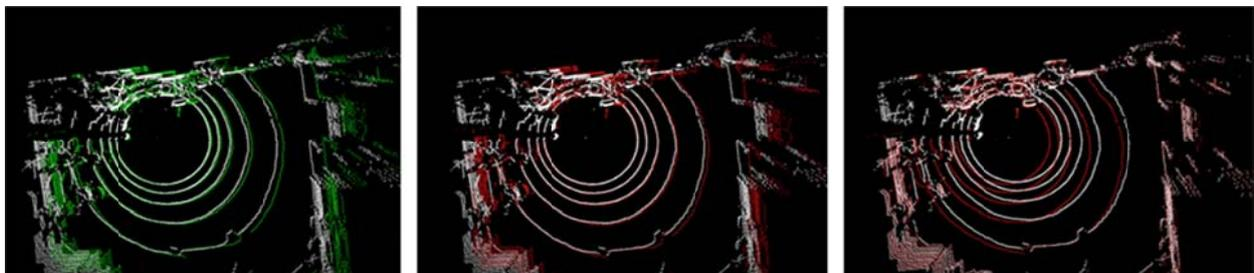
**Fig. 2** ICP results. White points of all images are original points and green and red points are target points. The left is the before the ICP algorithm. The middle is the results of the ICP algorithm without normal vector. The right is the results of the ICP algorithm considering the normal vector.
