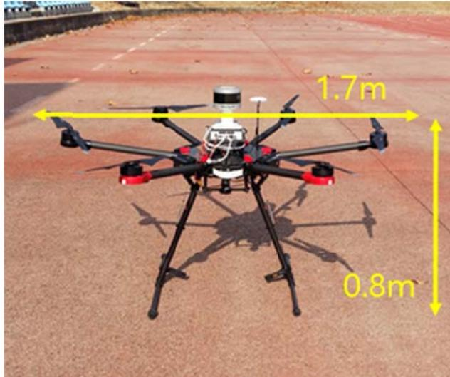
**Fig. 3** UAV sensor system. It is composed the UAV, single camera, 3D Lidar, RTK-GPS and mini PC.
