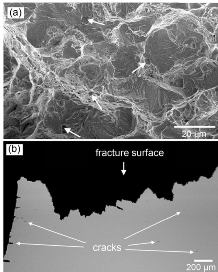
Fig. 1 SEM images of hydrogen-precharged super duplex stainless steel tensile tested at room temperature. (a) SEM image of the fracture surface. (b) SEM image of the longitudinal section near the fracture surface.
