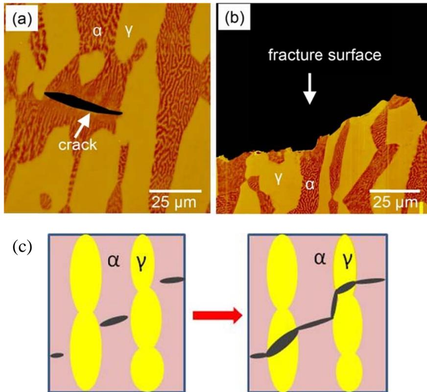
Fig. 2 MFM images of the longitudinal section of hydrogen-precharged super duplex stainless steel tensile tested at room temperature. (a) MFM image of a microcrack formed in the bulk. (b) MFM image of the section of fracture surface. (c) Illustration of macromechanism for hydrogen-assisted fracture in super duplex stainless steel.
