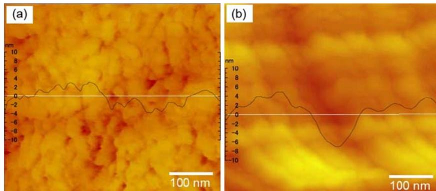
Fig. 3 STM images taken from the facets. (a) Nanoscale dimples. (b) Quasi-periodic corrugation. The inserts show the sectional profiles along the white lines.
