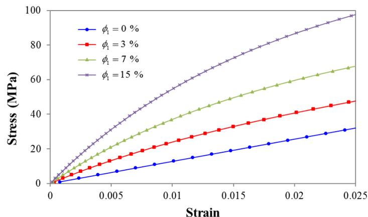
Figure 1. The predicted stress-strain behaviors composites with respect to the volume fraction of carbon fiber
