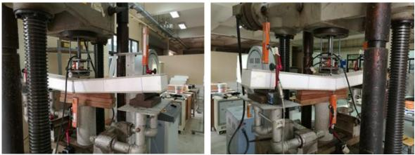
Fig. 3 Flexural collapse of test specimens
