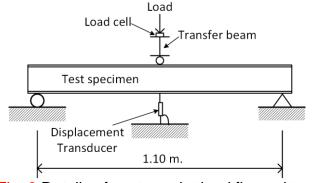
Fig. 2 Details of centre point load flexural test
