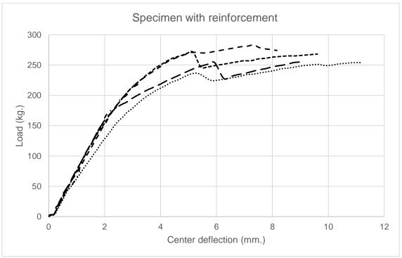
Fig. 5 Flexural behaviour of specimens with reinforcement
