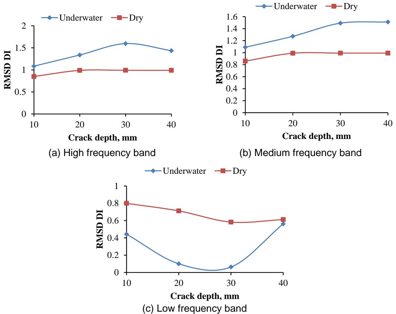
Fig. 4 Relationship between DI and crack depth for different frequency bands
