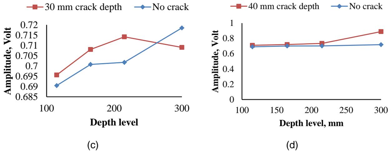
Fig. 3 Water pressure effect on amplitude of ultrasonic waves for different crack depth
