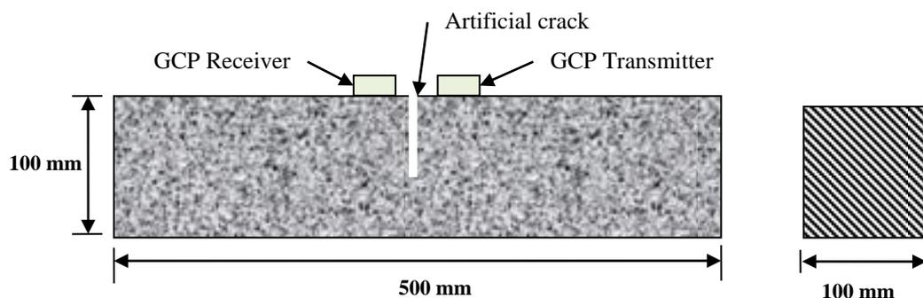
Fig. 1 Concrete beam layout showing sensors setup
