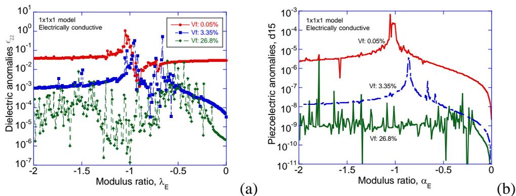
Fig. 3 (a) Effective dielectric constant, and (b) effective piezoelectric constant of the 1x1x1 composite model.
