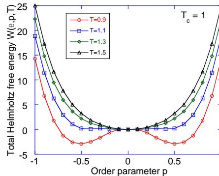
Fig. 1 Energy landscape of the 1D model with respect to spontaneous strain  $p$
