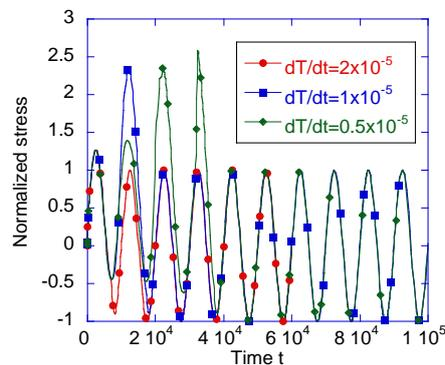
Fig. 3 Stress responses of the 1D system under sinusoidal displacement control with thermal cycling.
