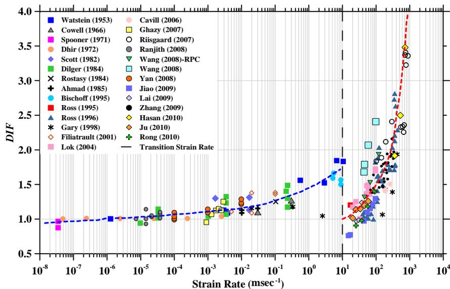
Fig. 3 Strain rate effect on compressive strength of concrete (updated from Pajak, 2011)
