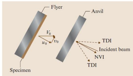
Fig. 2 Schematic of pressure-shear plate impact techniques (Sharpe, 2008)
