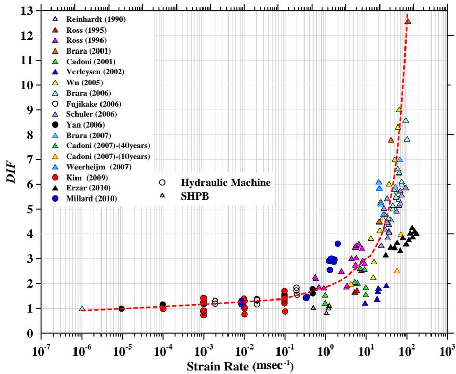
Fig. 4 Strain rate effect on tensile strength of concrete (updated from Pajak, 2011)
