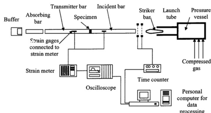
Fig. 1 Schematic configuration of split Hopkinson pressure bar system (Lok and Zhao, 2004)
