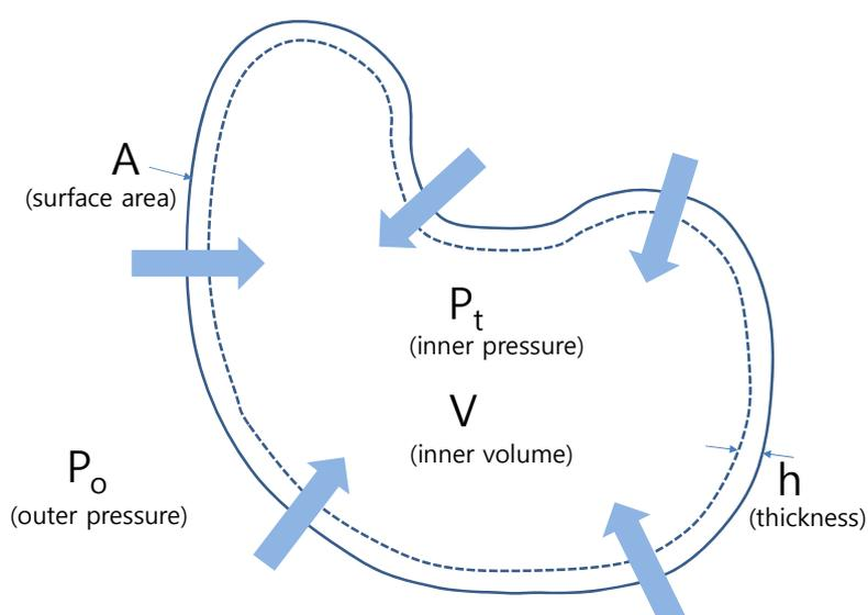
Fig. 1 Flow of fluid into a closed structure due to pressure drop
