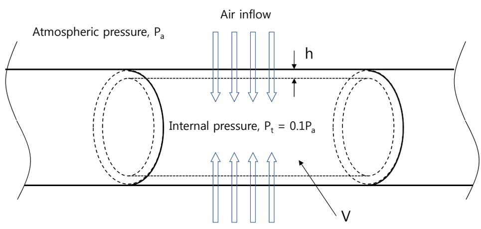
Fig. 2 Inflow of air into tube structure for SSTT
