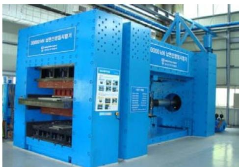
Fig. 1 30,000kN experimental equipment
