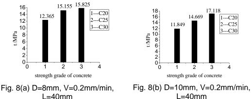
Fig. 8 Effect of strength grade of concrete on bond strength
