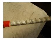
Fig. 4 The ribs stripping GFRP bars
