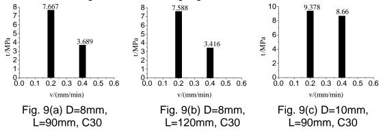
Fig. 9 Effect of loading speed on bond strength
