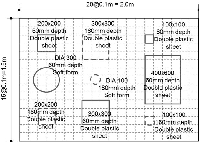
Fig. 5 The 2.0m × 1.5m reinforced concrete slab; The position of near-surface delamination defects are indicated with bold solid lines, those of deep delamination by bold dashed lines. The testing grid is indicated with light dashed lines
