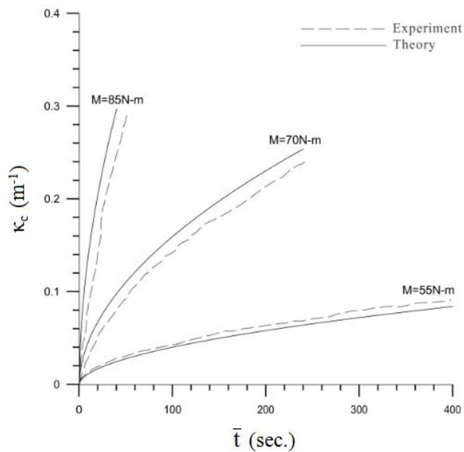
**Fig. 15** The experimental and simulated  $\kappa_c$ - $\bar{t}$  curves for sharp-notched SUS 304 stainless steel tubes with  $a = 0.8$  mm under pure bending creep in the initial and secondary stages
