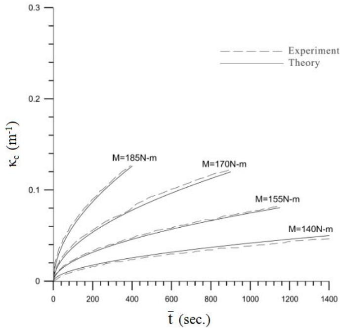
**Fig. 12** The experimental and simulated  $\kappa_c$ - $\bar{t}$  curves for sharp-notched SUS 304 stainless steel tubes with  $a = 0.2$  mm under pure bending creep in the initial and secondary stages
