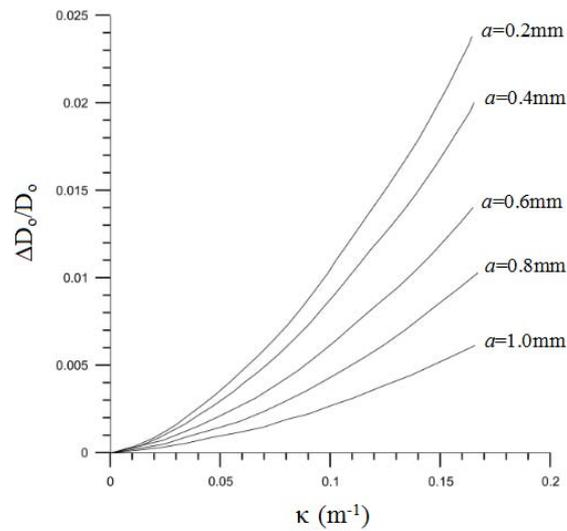
**Fig. 6** The corresponding experimental ovalization ( $\Delta D_o/D_o$ ) - curvature ( $\kappa$ ) curves for sharp-notched SUS 304 stainless steel tubes with different  $a$  under pure bending
