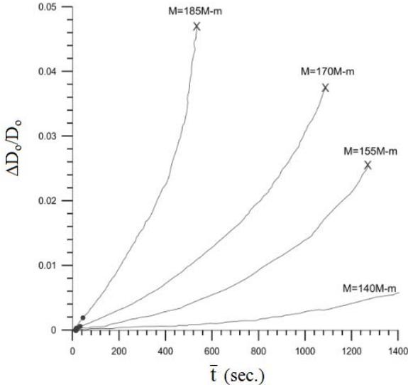
Fig. 9 The corresponding experimental ovalization ( $\Delta D_0/D_0$ ) – time ( $\bar{t}$ ) curves under pure bending and subsequent pure bending creep for Fig. 7
