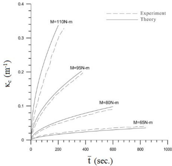
**Fig. 14** The experimental and simulated  $\kappa_c$ - $\bar{t}$  curves for sharp-notched SUS 304 stainless steel tubes with  $a = 0.6$  mm under pure bending creep in the initial and secondary stages
