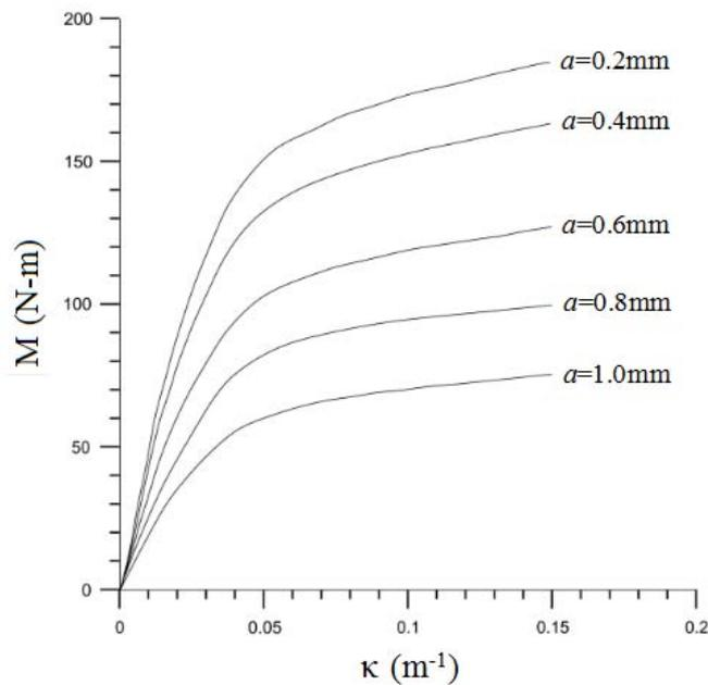
Fig. 5 The experimental moment ( $M$ ) - curvature ( $\kappa$ ) curves for sharp-notched SUS 304 stainless steel tubes with different  $a$  under pure bending
