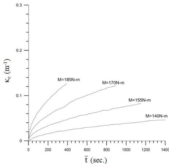
Fig. 10 The experimental  $\kappa_c$ - $\bar{t}$  curves for sharp-notched SUS 304 stainless steel tubes with  $a = 0.2$  mm under pure bending creep in the initial and secondary stages
