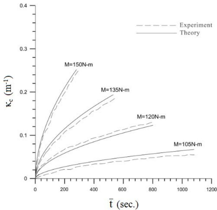
**Fig. 13** The experimental and simulated  $\kappa_c$ - $\bar{t}$  curves for sharp-notched SUS 304 stainless steel tubes with  $a = 0.4$  mm under pure bending creep in the initial and secondary stages
