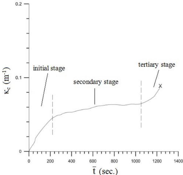
Fig. 8 The creep curvature ( $\kappa_c$ ) – time ( $\bar{t}$ ) curve with the held moment of 155 N-m
