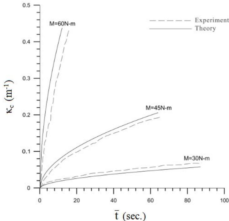
**Fig. 16** The experimental and simulated  $\kappa_c$ - $\bar{t}$  curves for sharp-notched SUS 304 stainless steel tubes with  $a = 1.0$  mm under pure bending creep in the initial and secondary stages
