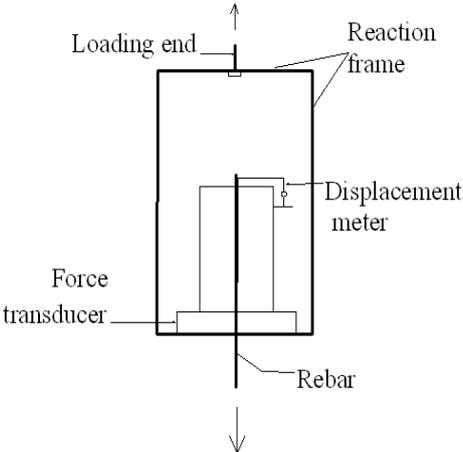
**Fig.1 Schematic Representation of Pull-out Test Setup**
