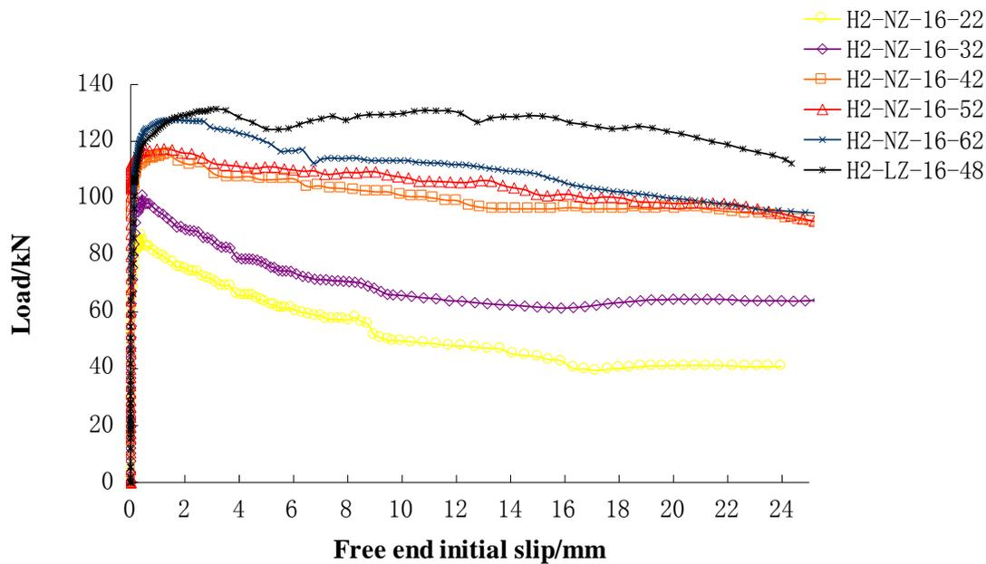
**Fig.4 Load slip curves for different thicknesses of protective layer**
