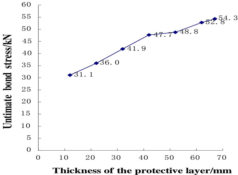
**Fig.5 Ultimate bond stress - protective layer relationship**
