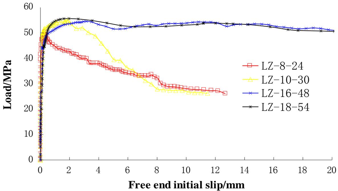
Fig. 6 Varying diameters bond-slip curves
