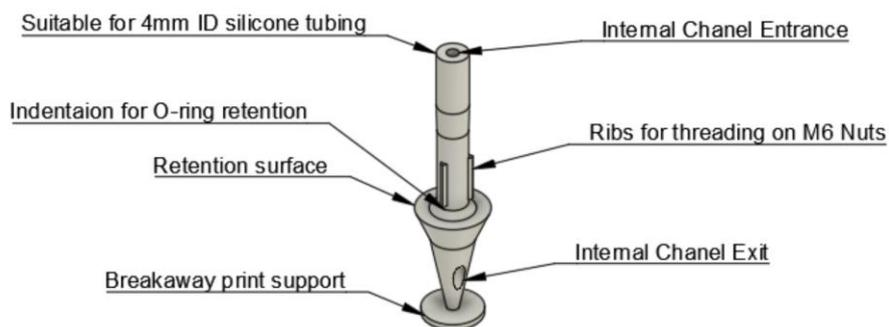
Fig. 2 Single use fitting design.
