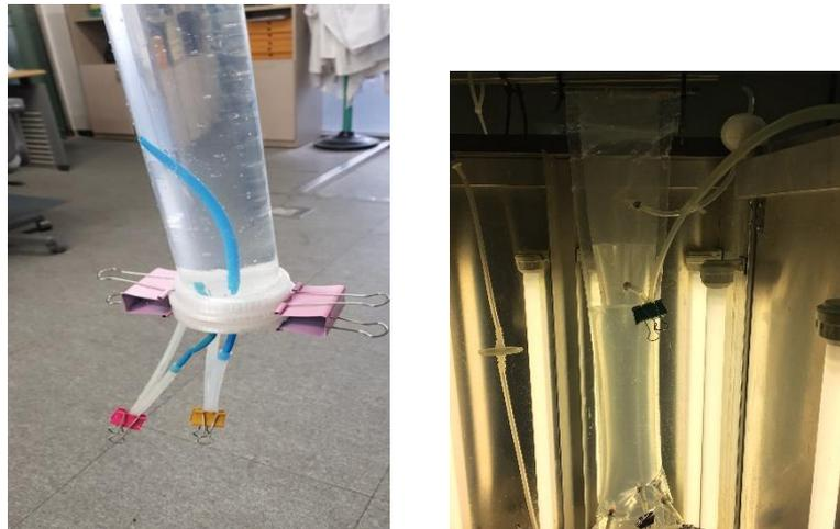
Fig. 4 Fitting clamped fitting for multi use bags (left) and bag in bag reactor with single use fittings (right).
