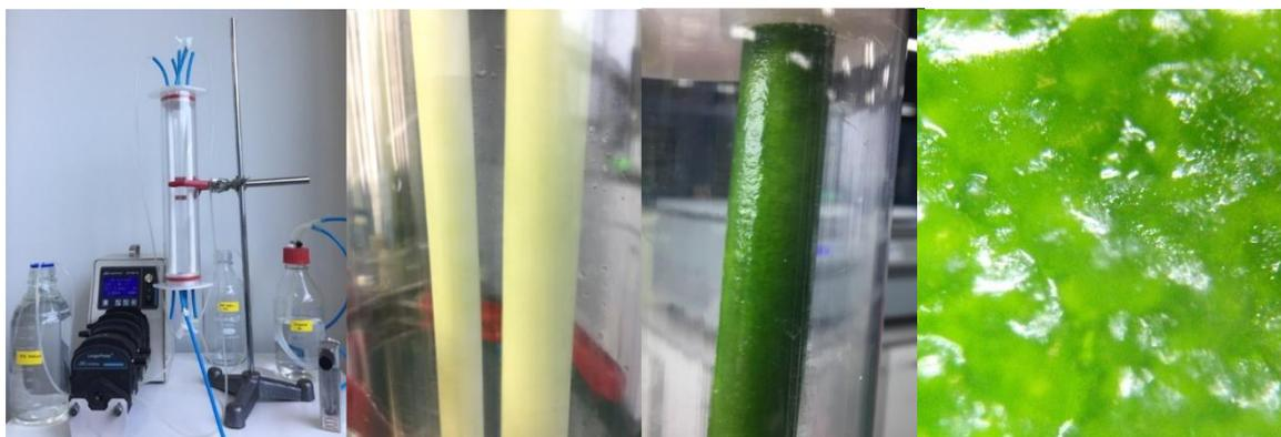
Fig. 5 from left to right: Biofilm reactor from acrylic pipe, porous tubes of expanded UHMW PE and 3D printed fittings, Biofilm at day 1, Biofilm at day 36 and close up of cultivated biofilm of *Chlamydomonas asymmetrica* after cultivation for 36 days at 100x magnification.
