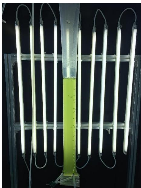
Fig. 3 Single use bag reactor with 3D printed fittings.
