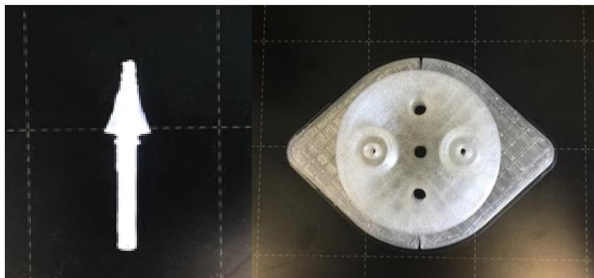
Fig. 1 Single use fitting (left) and multi use fitting (right) 3D printed from ABS.
