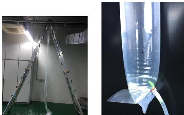
Fig. 8 Leak test for 65mm ID, 70µm wall thickness hanging bag (left) and leak test for 3D printed single use fitting inserted into 70µm wall thickness PE bag (right).
