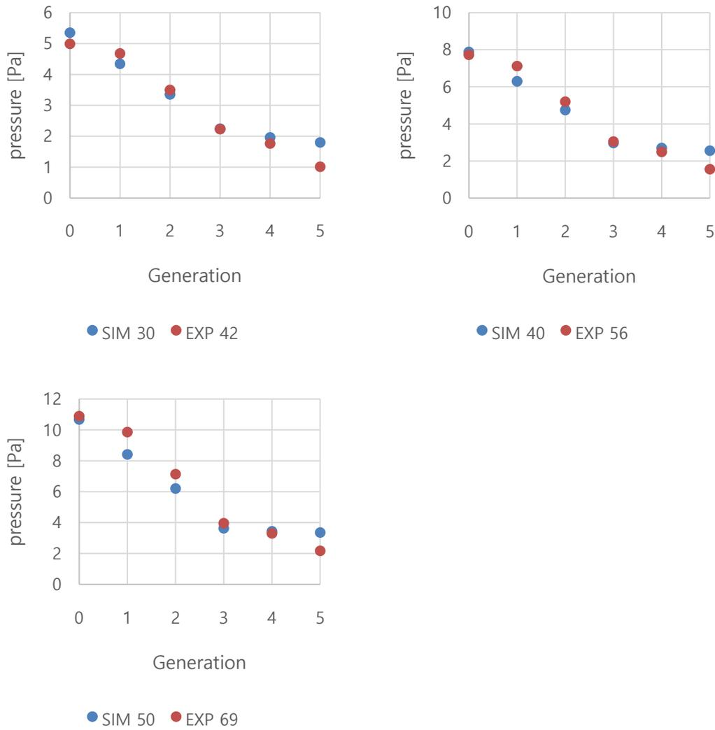
Fig. 3 Pressure in generation 0 to 5 for the volume flow combinations: simulation 30 l/min experiment 42 l/min, simulation 40 l/min experiment 56 l/min, simulation 50 l/min experiment 69 l/min
