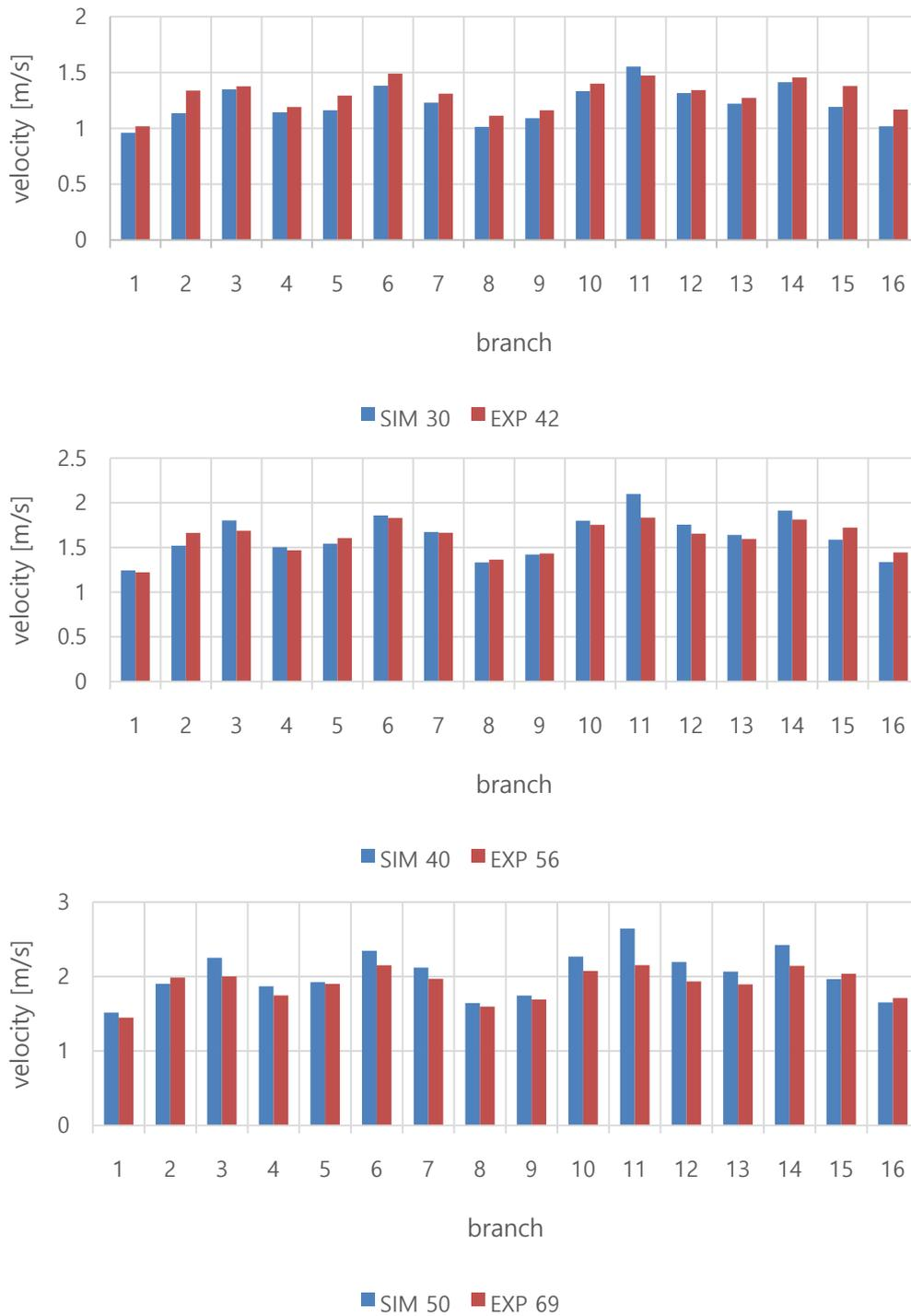
Figure 4 Velocity distribution in generation 5 for the volume flow combinations: simulation 30 l/min experiment 42 l/min, simulation 40 l/min experiment 56 l/min, simulation 50 l/min experiment 69 l/min
