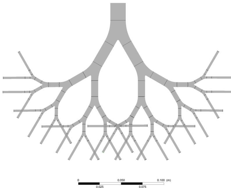
Fig. 1 Geometry of the numerical lung model
