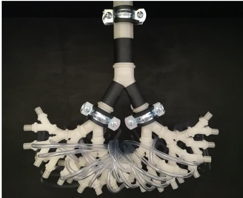
Fig. 2 Experimental lung model
