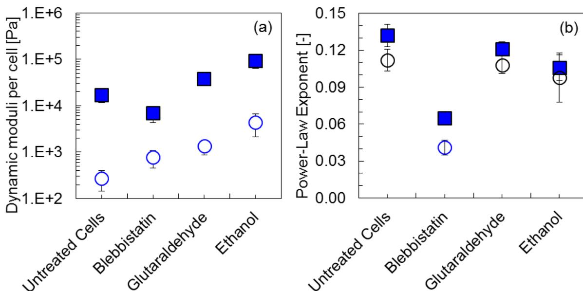
Fig. 3 Dynamic moduli per cell (a) and power-law exponent (b) for untreated fibroblasts and fibroblasts treated with different drugs. The storage modulus, the loss modulus and their respective exponents are indicated by closed and open symbols, respectively. Frequency in (a): 1 Hz; amplitude in (b): 0.2%; gap width: 5  $\mu$ m.
