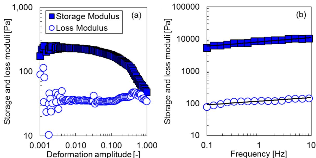
Fig. 2 Amplitude sweep at a gap width of 10  $\mu\text{m}$  at a frequency of 1 Hz (a) and frequency sweep at a gap width of 5  $\mu\text{m}$  and a strain amplitude: 0.2% (b). Storage modulus and loss modulus are indicated by closed and open symbols, respectively.
