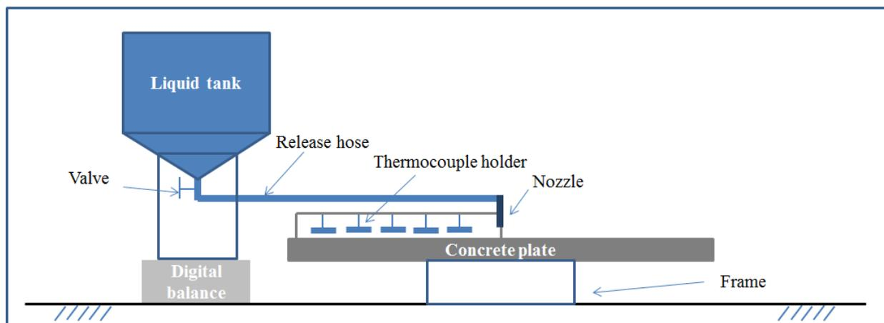
**Fig. 2** General schematic layout of the experimental apparatus
