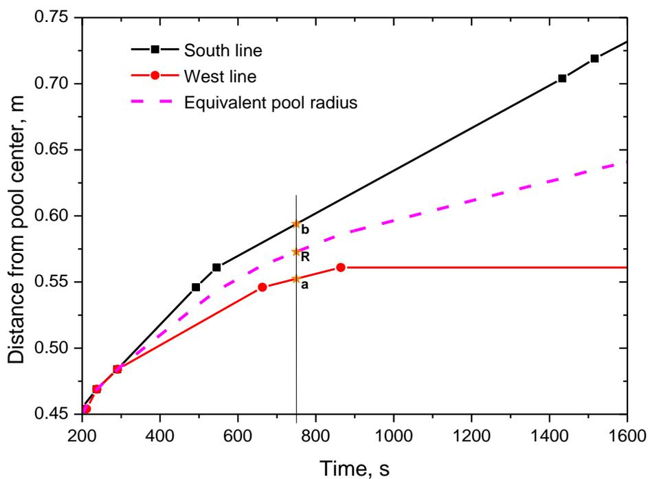
Fig. 5 Equivalent radius for the 6 mm nozzle
