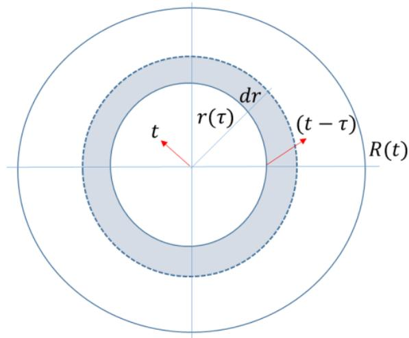
**Fig. 1** Vaporization from the spreading pool
