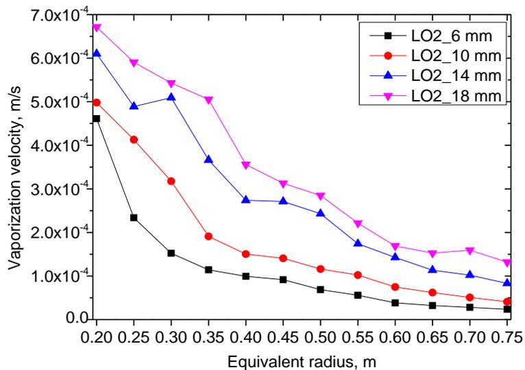
Fig. 9 Vaporization velocity versus pool radius for liquid oxygen
