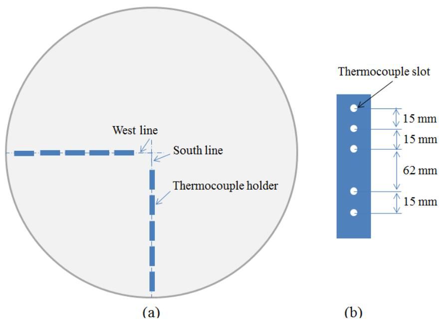
**Fig. 3** Thermocouple distribution (a) General schematics (b) Thermocouple holder's detail
