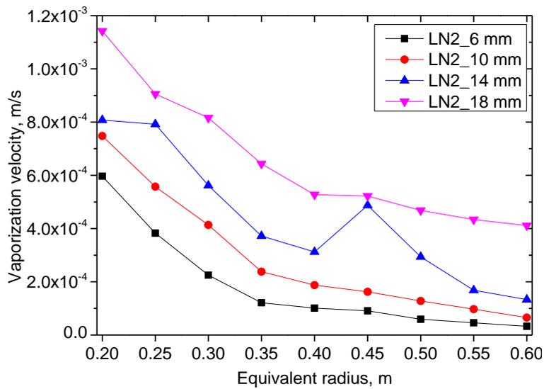
Fig. 8 Vaporization velocity versus pool radius for liquid nitrogen
