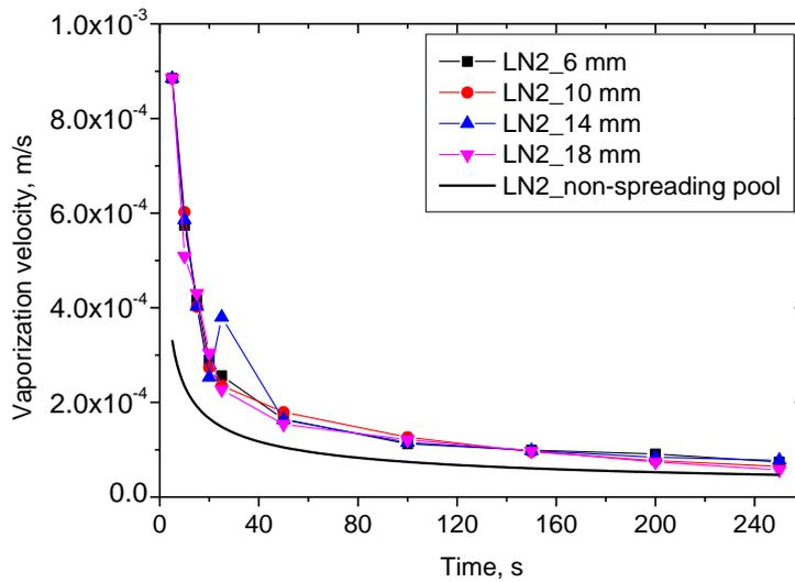
Fig. 10 Vaporization velocity versus time for liquid nitrogen
