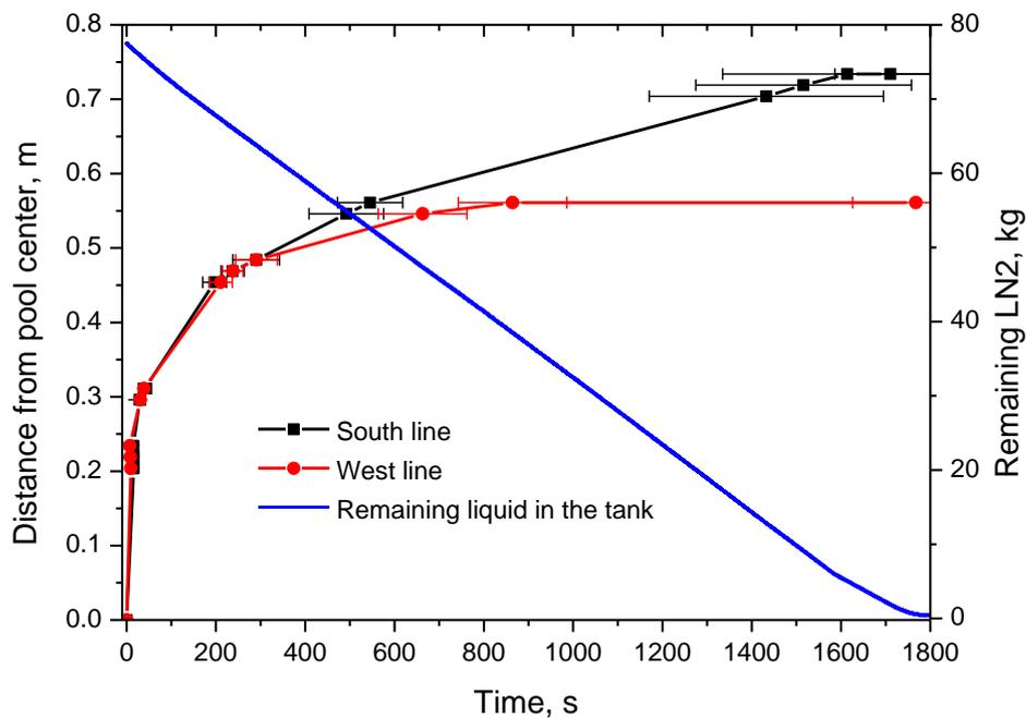
**Fig. 4** Spread data for the 6 mm nozzle
