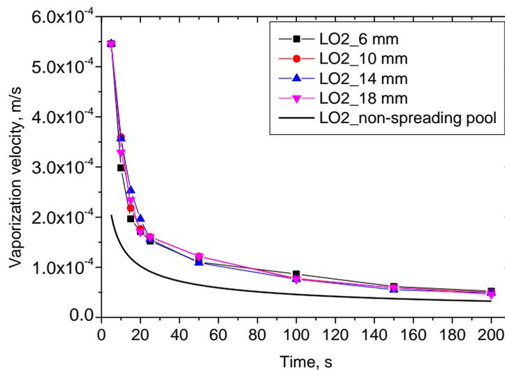
Fig. 11 Vaporization velocity versus time for liquid oxygen
