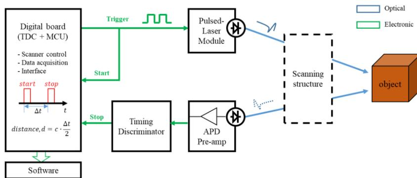
Fig. 3 Principle of the pulsed time-of-flight LiDAR
