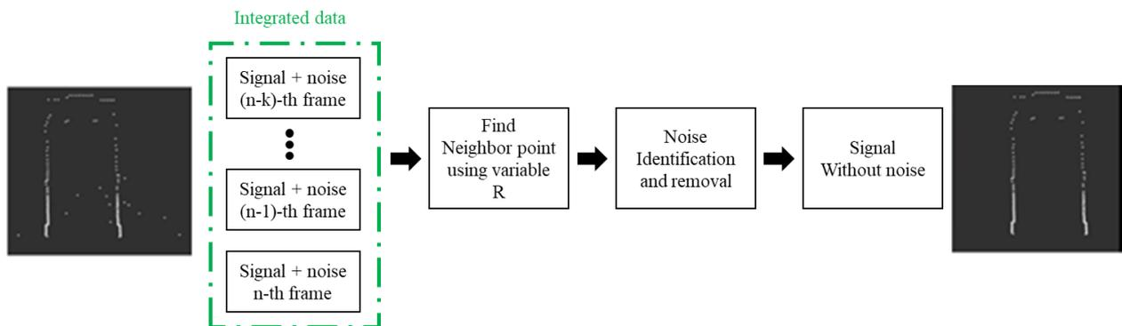
Fig. 6 The adaptive radius outlier removal algorithm
