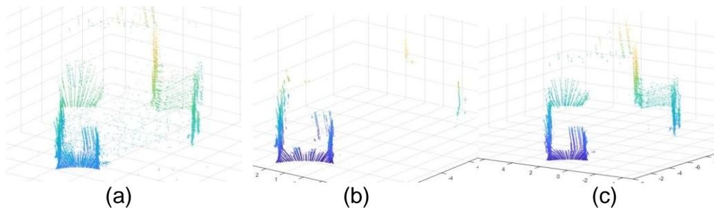
Fig. 7 The adaptive radius outlier removal algorithm filtering result, (a) LiDAR data with simulated noise (b) ROR (c) Adaptive ROR
