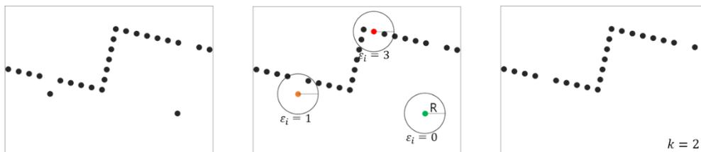
Fig. 2 radius outlier removal method
