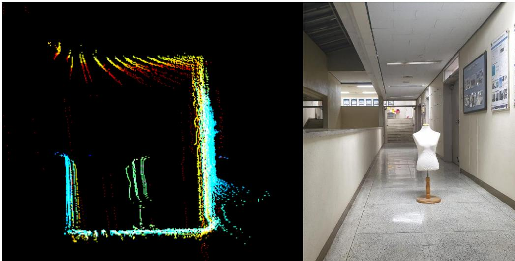
Fig. 5 The measurement result of designed 3D LiDAR
