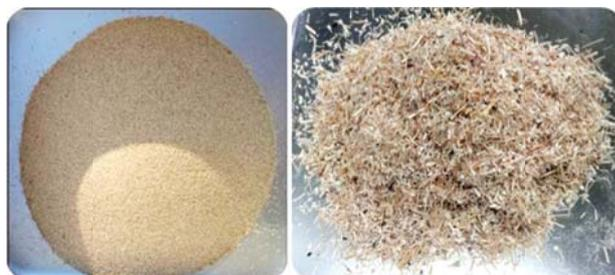
Fig. 2 Standard silica sand (left) and sawdust of wood larch (right)
