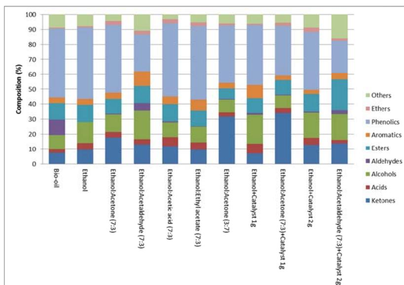
Fig. 1 GC-MS analyses of pyrolysis oil and upgraded pyrolysis oil
