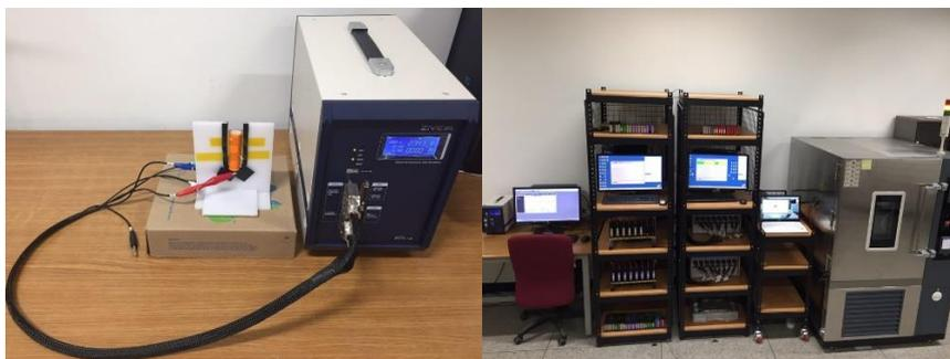
Fig. 2 Electrochemical and electrical set for test of Li-ion cells
