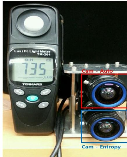
Fig1. Camera configuration for exposure control
