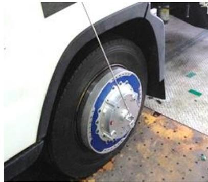
Fig. 5 Installation WFT on the vehicle and measuring wheel weight using scale
