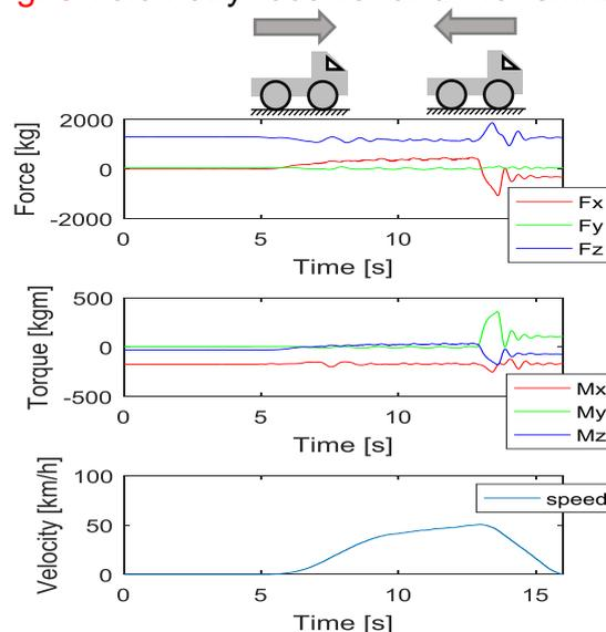
Fig. 7 Driving test of WFT with 2.5 ton truck. WFT is installed left-front wheel. Vehicle accelerate for 10s and brakes at 13s.
