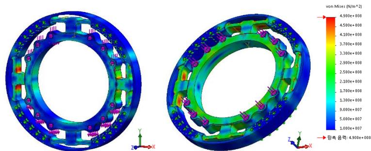
**Fig. 2** FEM analysis of WFT structure
