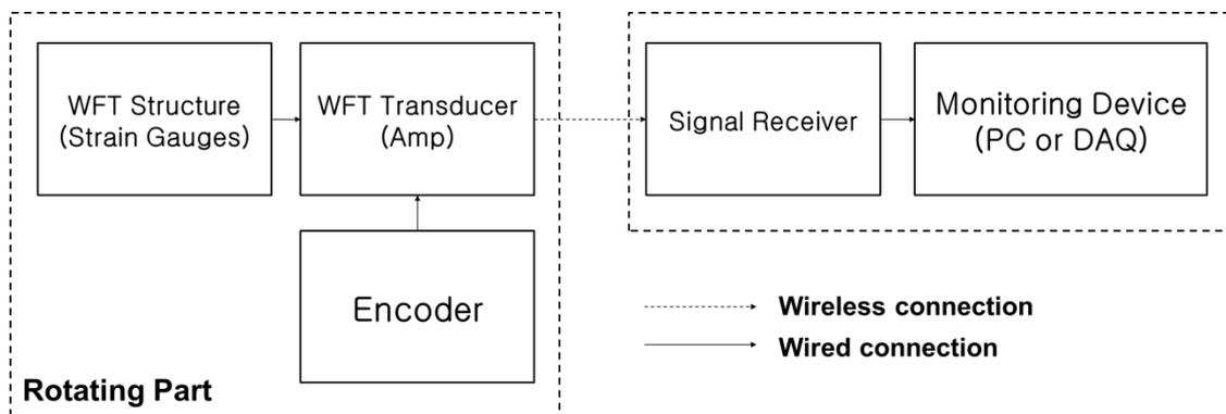
**Fig. 4** WFT signal processing block diagram
