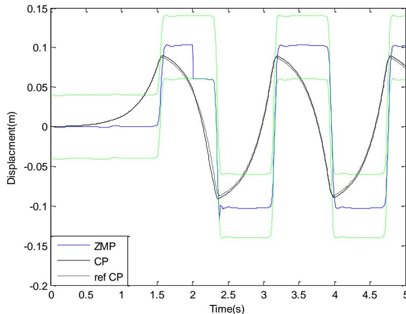
Figure 1 Simulation result of a proposed walking pattern under the small disturbance
