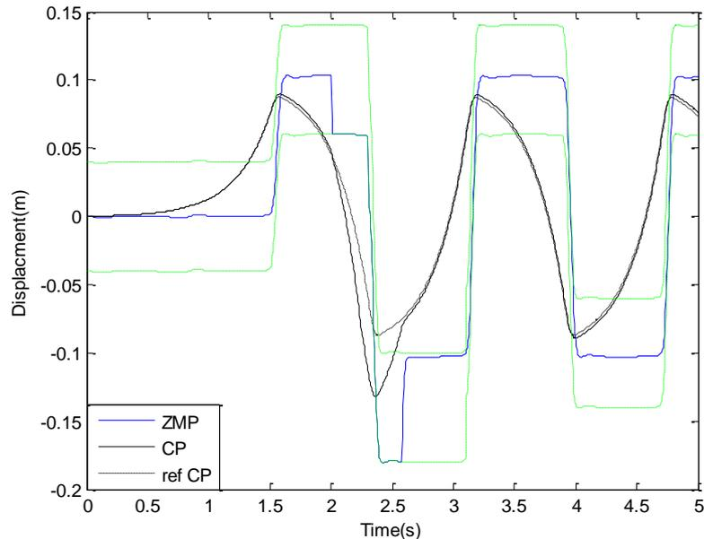
Figure 2 Simulation result of a proposed walking pattern under the large disturbance
