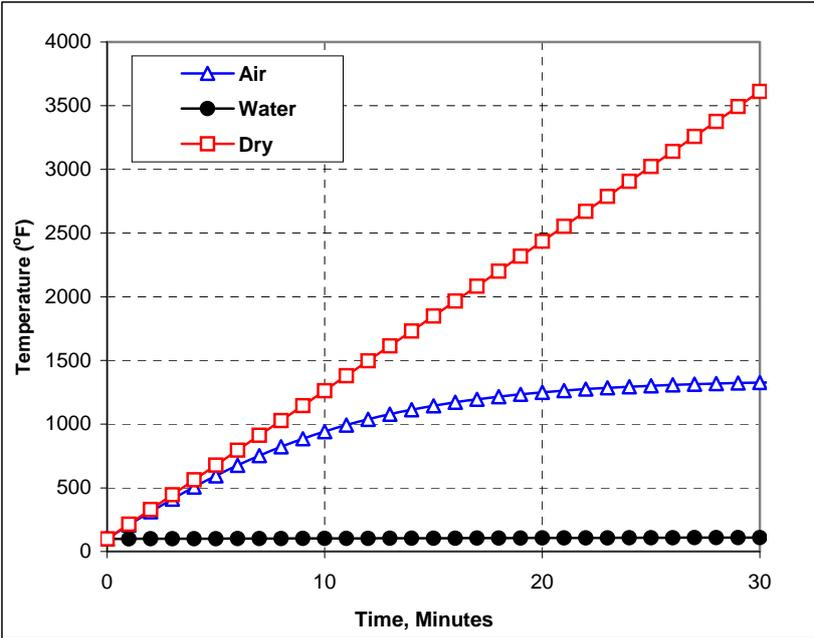
Figure 5 - Influence of different medium on bit temperature.
