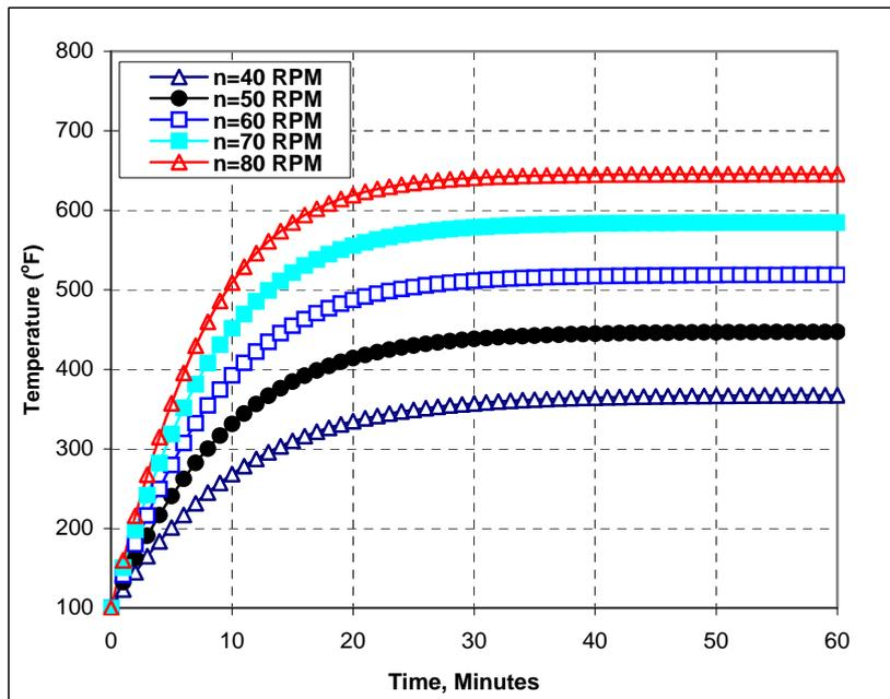
**Figure 7 - Influence of rotary speed on bit temperature.**
