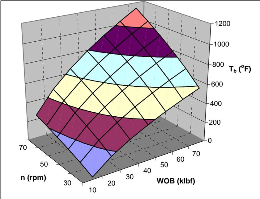
**Figure 8 - Determination of weight on bit and rotary speed.**
