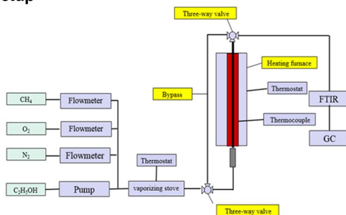
Fig. 1. Experimental schematic of Ethanol pyrolysis
