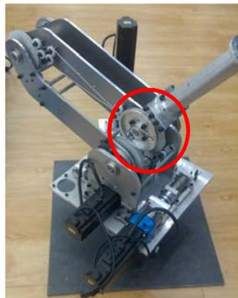
Fig. 1 The newly designed cable-driven manipulator “Polaris-I” without last 3-DOFs
