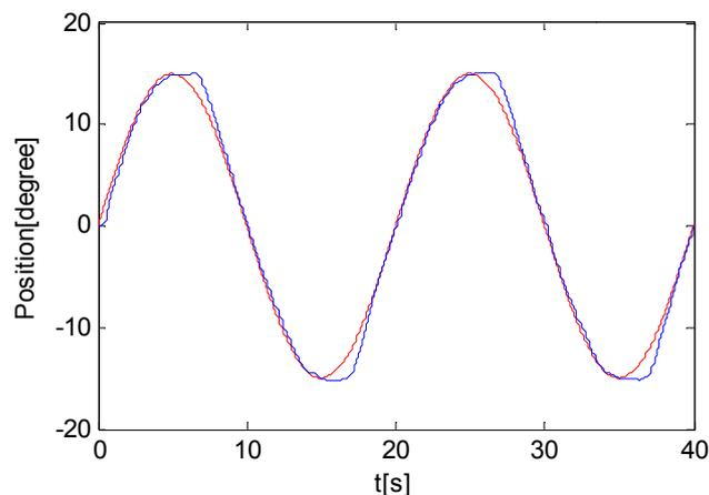
Fig. 2 Trajectory tracking performance: red solid (desired) vs blue solid (actual);
