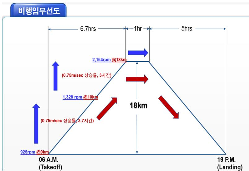
Fig. 4 Simplified flight mission profile of EAV-3
