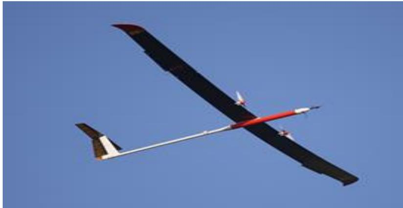
Fig. 2 Flight test of EAV-2H, twin propellers
