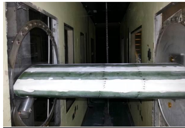
Fig. 2 The clean DU91-W2-250 airfoil, showing 3 of the 5 inserts where actuators will later be installed, in the Knapp-Meadow wind tunnel of Tel Aviv University. Chord c=480\text{mm} .
